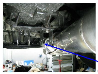
Install OEM hanger with spring here
