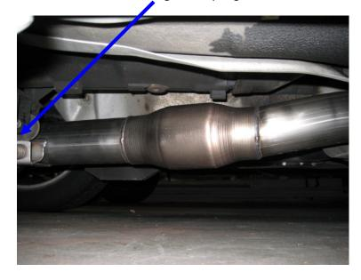
Clean photo of new hardware, before OEM hanger is bolted in place. (thanx Shawn)
