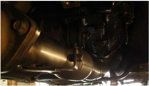
Support the back end of Section #2, while the rear section #3 is installed
