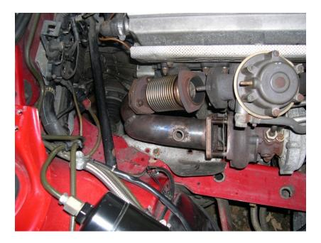
**5**: Catalytic section Installation: Be certain that the installer places the front most hanger on the transmission according to the following photos. Failure to do this will cause premature failures that void warranty.
